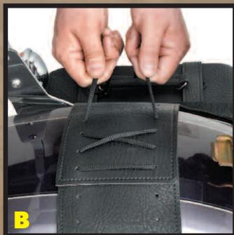
Warning: Saddlebags must never contact the rear wheel, drive train, suspension or exhaust. A minimum clearance of two (2) inches, with the suspension compressed, is
