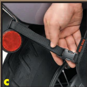
Connect the quick-release buckles and pull the adjustment straps tight. This secures each half saddlebag to your motorcycle. Because our bags fit a number of styles and sizes of motorcycles, we do not have specific places we recommend to secure the straps to your bike.
