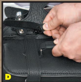
Warning: If the male zipper starter is not fully inserted into the zipper pull (slider), the zipper will disconnect, and the saddlebag will detach from the mounting yoke.
